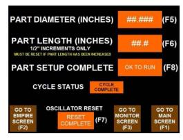
event that the new part to be run is Longer than the previous part, the oscillator will need to be reset by either pressing the "F7" button or the "reset" button on the screen.
