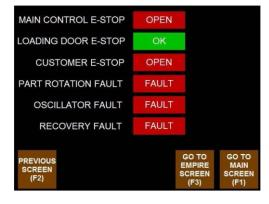
the event that they fall outside of their tolerance range for more than 5 seconds, a fault will be generated and the cycle will be put on hold.
