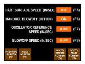
"OSCILLATOR REFERENCE SPEED" sets the reference value used to calculate the horizontal travel speed of the BLAST OSCILLATOR during a cycle. This is also the speed that the largest diameter part would be run at. The actual Oscillator speed is the ratio of the largest part diameter / the current part diameter multiplied by this reference value. "BLOWOFF SPEED" is the travel speed of the BLAST OSCILLATOR during its BLOWOFF stroke, return to home.
